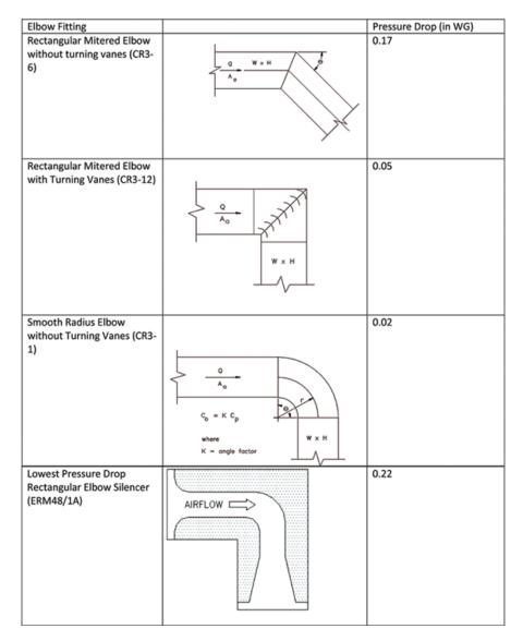
Claims of an elbow silencer having pressure drop comparable to a smooth radius elbow would be questionable at best and need to be substantiated and proven.
